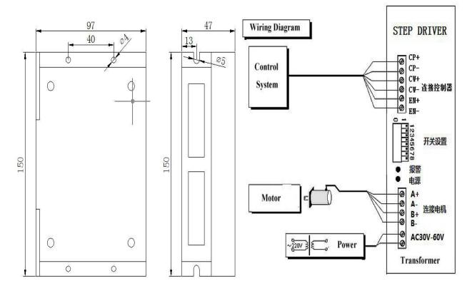
This driver sets the number of microstep and phase currents by dial switch. According to the label set: high number of microstep motors run more smooth when the control frequency allows; specific settings refer to the following table (ON = 0, OFF = 1):
